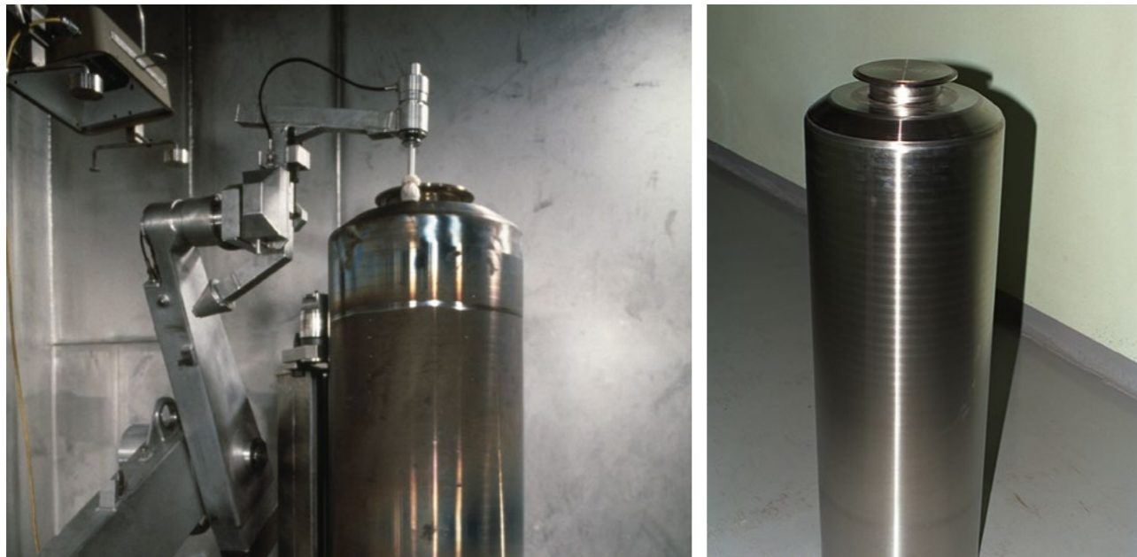
Figure 12: Loading of a cask with HAW canisters (left), single canister (right)
